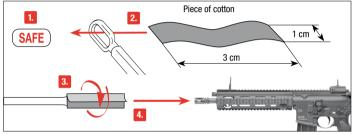
Put the safety on "safe". Prepare a thin rod with a length of approx. 30 cm. Attach a piece of cotton fabric to its end and clean the barrel with some silicone oil.
